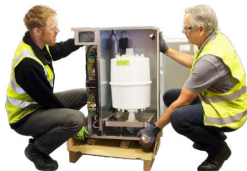
Fig 2c - Lifting the unit, front panel removed
